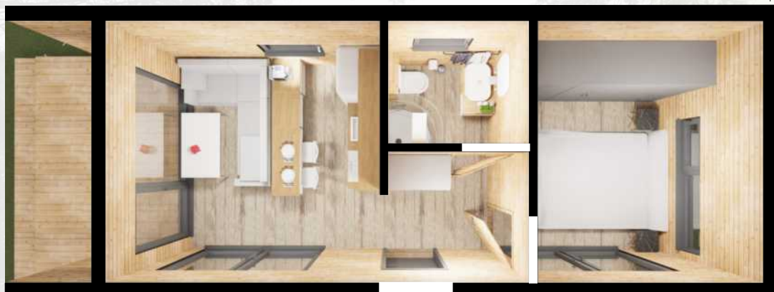
Architectural floor plan of a kitchen and living area. The plan shows a kitchen with a sink, stove, and refrigerator, a living area with a sofa and coffee table, and a bedroom with a double bed. Dimensions are provided for various elements and overall room sizes. Labels and dimensions: WYPOCZYNEK ROZKŁADANY (Expandable sofa) - 145 ZABUDOWA KUCHENNA (Kitchen unit) - 175 ŁODÓWKI ZABUDOWA KUCHENNA (Kitchen unit with refrigerator) SZAFKA (Cabinet) - 265 STOLIK (Coffee table) - 200 SZAFKA (Cabinet) - 800 ŁÓŻKO PODWÓJNE (Double bed) - 265 Dimensions: 340 (total width), 206 (kitchen unit width), 104 (living area width), 104 (bedroom width), 310 (living area depth), 165 (bedroom depth), 310 (living area depth), 145 (sofa width), 175 (kitchen unit width), 104 (living area width), 104 (bedroom width), 200 (coffee table width), 265 (bed width), 800 (cabinet width).
